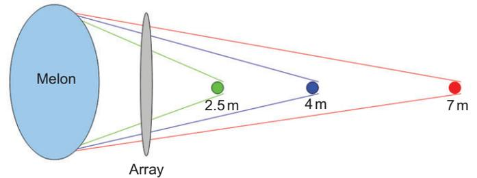
Fig. 7. Schematic of proposed focusing mechanism that would result in increased beam areas measured at the site of the array. Beam areas would appear to increase if the subject is adjusting her focal region according to the distance of the target.
