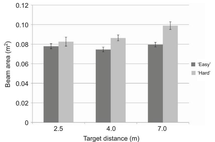
Fig. 5. Beam area ( $\text{m}^2$ ) according to target distance (m) and difficulty. The beam area represents the marginal mean beam area value across all frequencies for each target condition. Beam areas are larger for difficult targets and increase with increasing target distance. The error bars represent the standard error for each marginal mean value.
