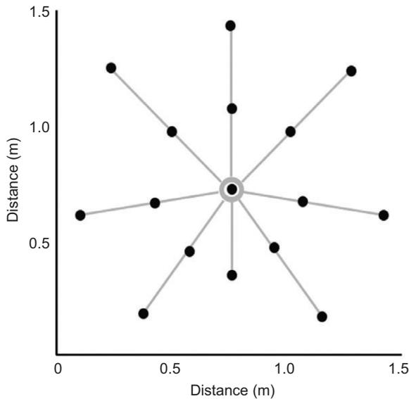
Fig. 2. Diagram and dimensions of the 16-element hydrophone array. Each solid black circle represents the location of a single hydrophone.
